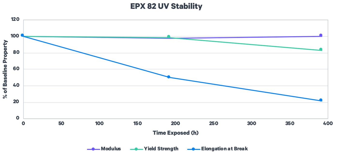
ASTM 4459: Q-Sun XE-1, 0.8 W/m<sup>2</sup> at 420 nm, 55 °C
