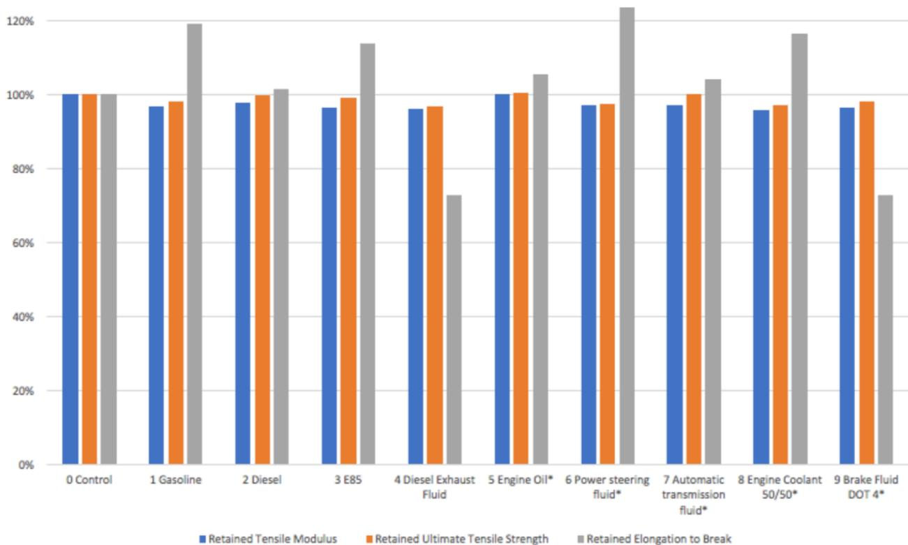
**Treatment Method:** Samples submerged in test liquid for 30 minutes at 23 °C or 50 °C (starred) then removed from test liquid and allowed to sit at ambient room temperature conditions for 1 week (samples were not wiped).
